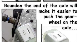
Put the motor in the gear and check the right position of the brass gearwheel.
